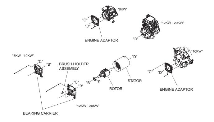
Figure 1. AC Generator Exploded View
